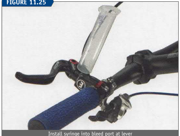
Install syringe into bleed port at lever
