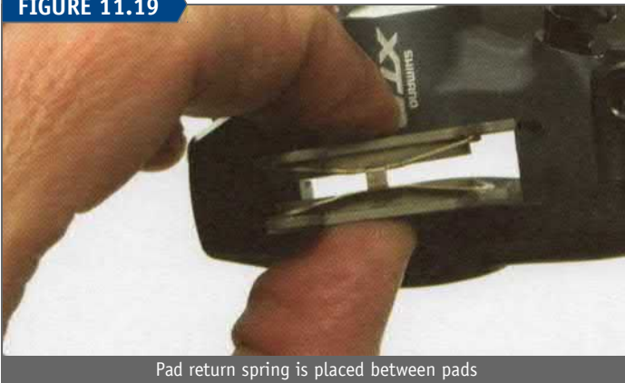
Pad return spring is placed between pads
