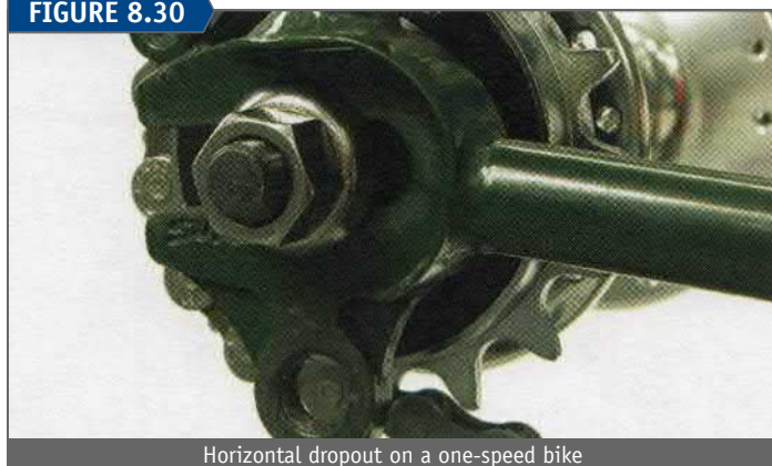
Horizontal dropout on a one-speed bike
