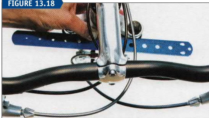
Stem is misaligned when bars are not parallel to fork blades
