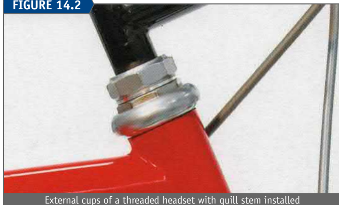
External cups of a threaded headset with quill stem installed
