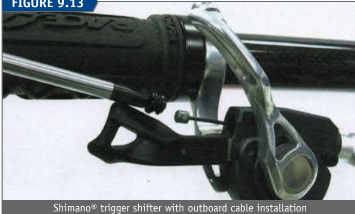
Shimano® trigger shifter with outboard cable installation
