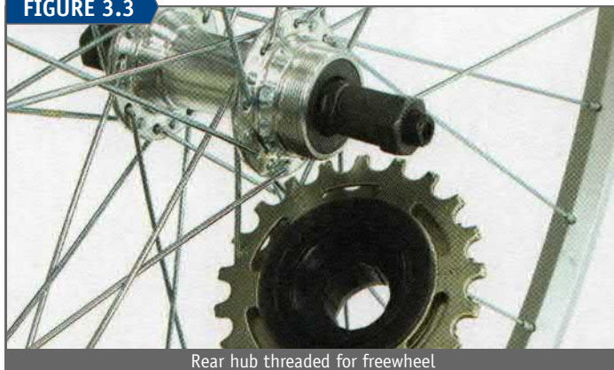
Rear hub threaded for freewheel
