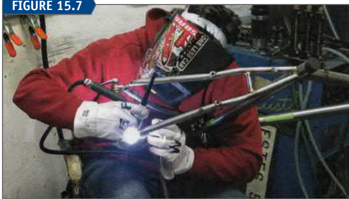
Welding of a steel frame (Photo credit Independent Fabrication®)
