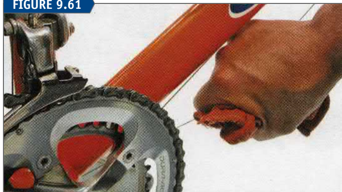
Pull cable by hand to isolate limit screw performance from index settings
