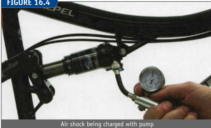
Air shock being charged with pump
