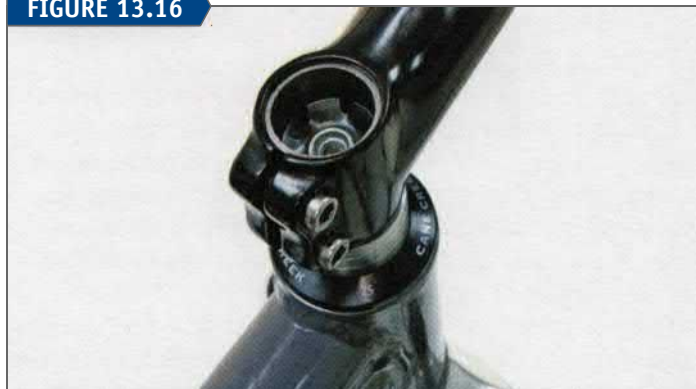
Threadless steering column recessed below threadless stem
