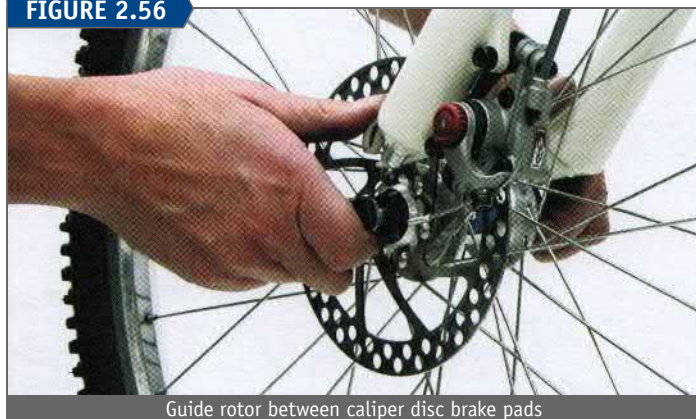
Guide rotor between caliper disc brake pads
