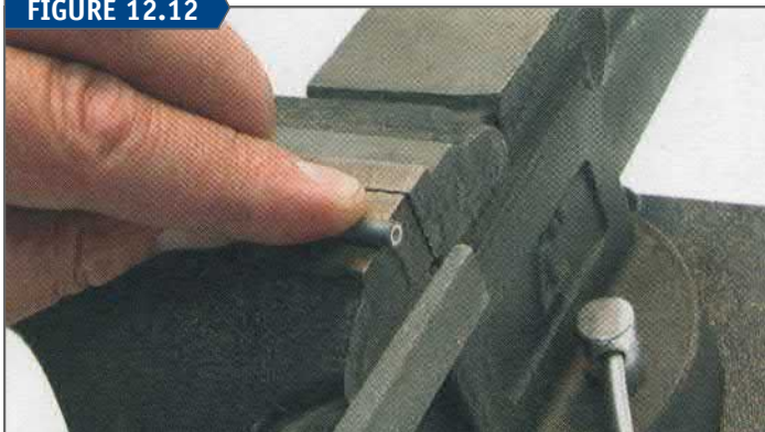
File brake coil smooth to eliminate burr from side cutters
