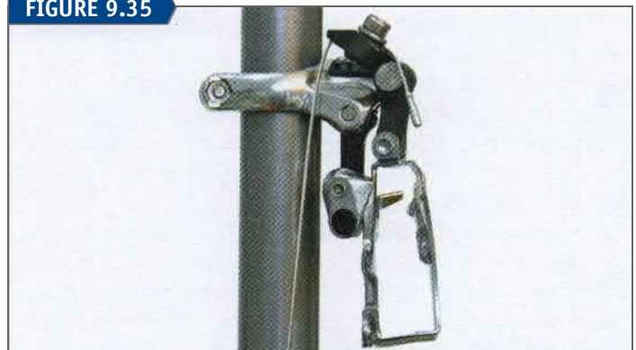
Bottom swing design with bottom cable pull
