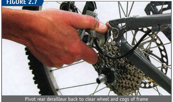
Pivot rear derailleur back to clear wheel and cogs of frame
