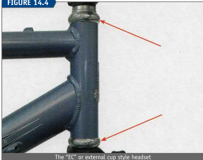
The "EC" or external cup style headset
