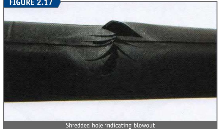
Shredded hole indicating blowout
