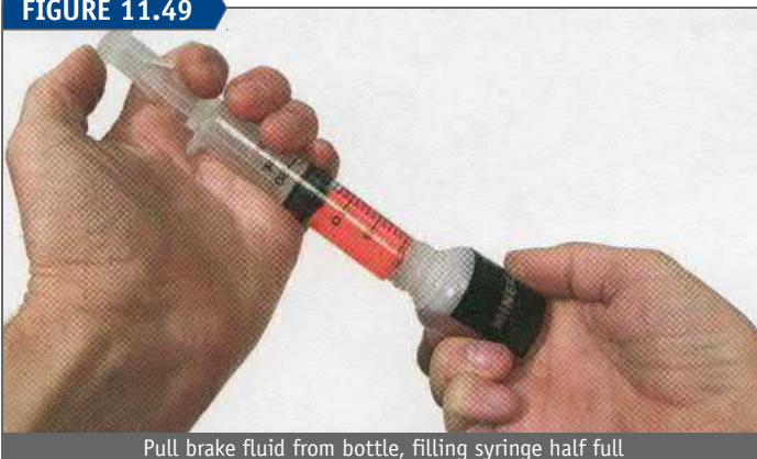
Pull brake fluid from bottle, filling syringe half full
