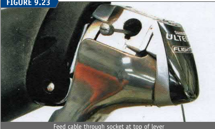
Feed cable through socket at top of lever
