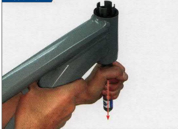
Draw the Race Tool RT-1 or RT-2 through headtube small side first
