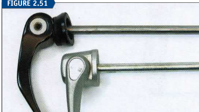
Open cam style seen on the top, and closed cam seen on the bottom
