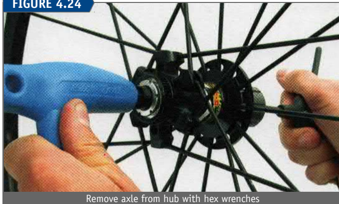
Remove axle from hub with hex wrenches
