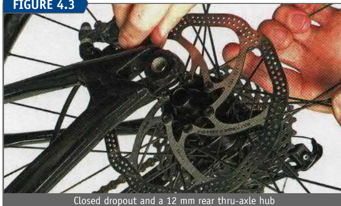
Closed dropout and a 12 mm rear thru-axle hub
