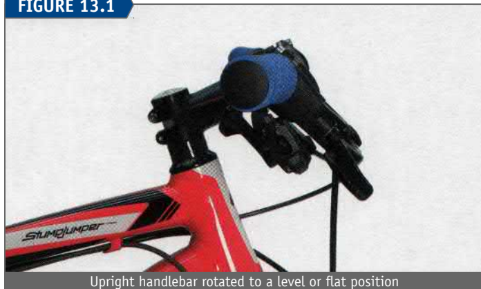
Upright handlebar rotated to a level or flat position
