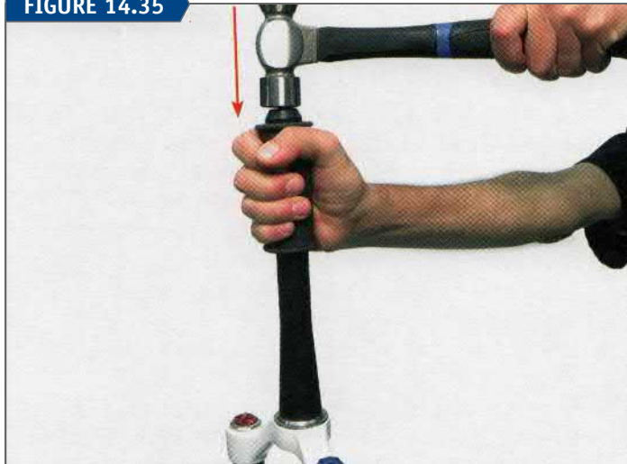
Drive the star nut down while guiding with the TNS-4
