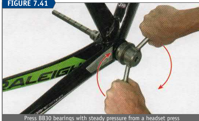
Press BB30 bearings with steady pressure from a headset press
