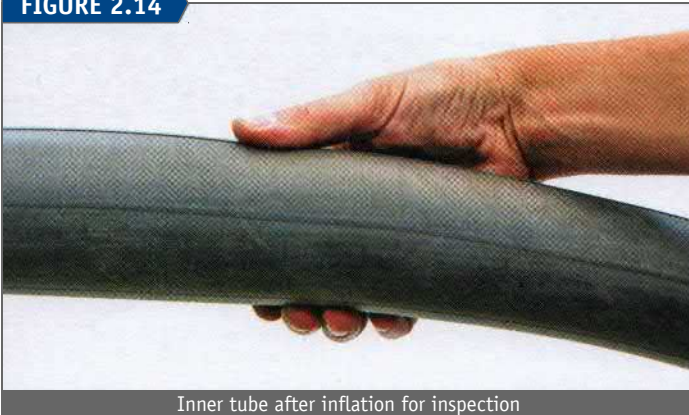
Inner tube after inflation for inspection
