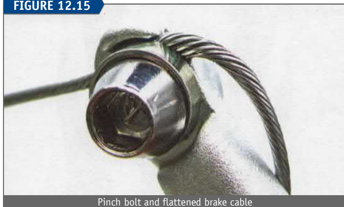
Pinch bolt and flattened brake cable
