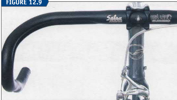
Housing enters stop in a straight line, indicating a good length
