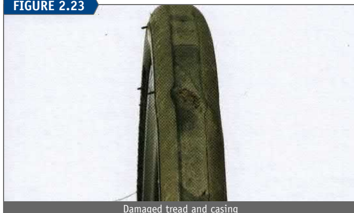
Damaged tread and casing
