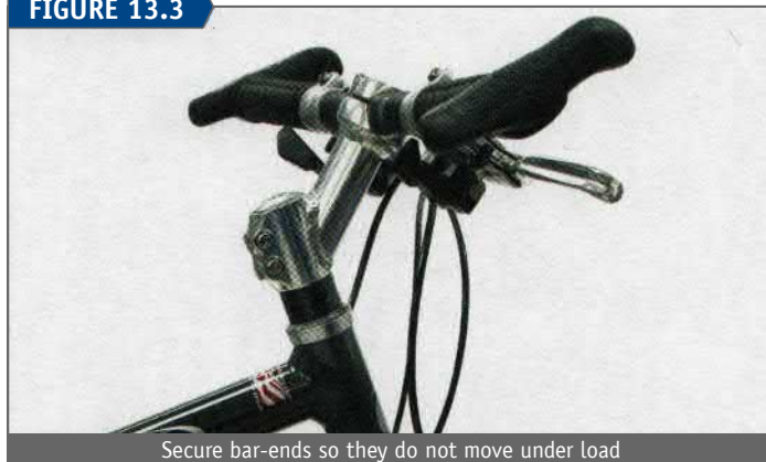
Secure bar-ends so they do not move under load
