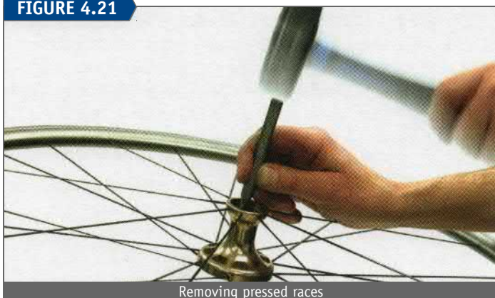
Removing pressed races
