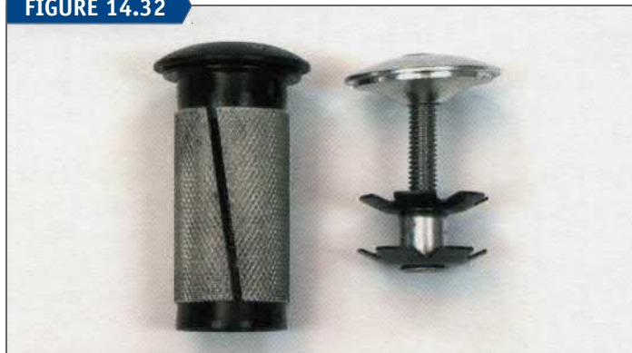
Compression plug on the left. Star nut with bolt and top cap on the right.
