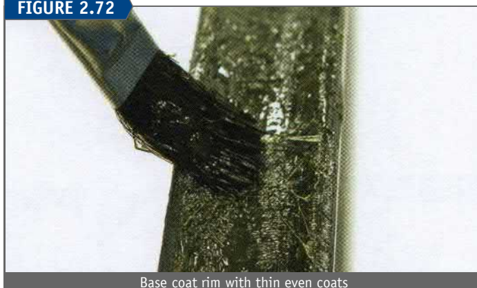
Base coat rim with thin even coats
