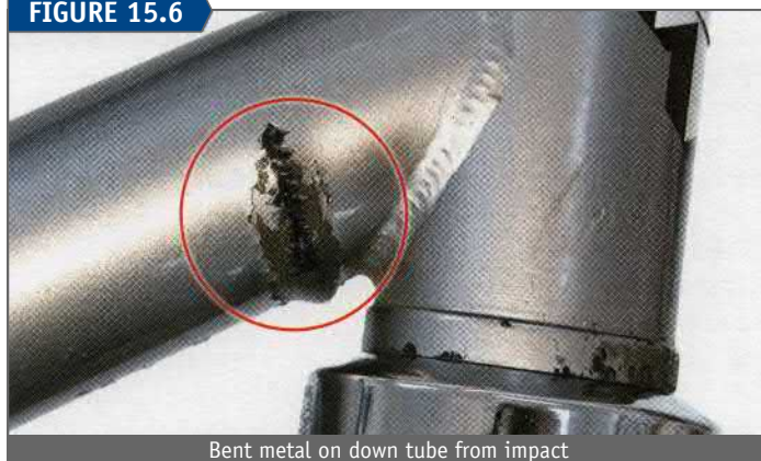
Bent metal on down tube from impact
