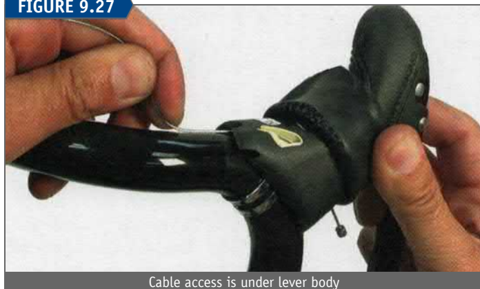
Cable access is under lever body
