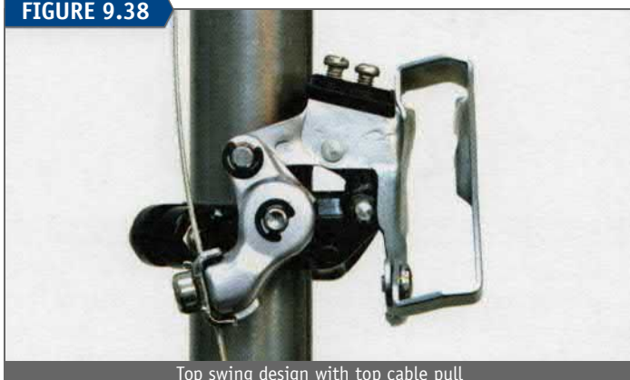
Top swing design with top cable pull
