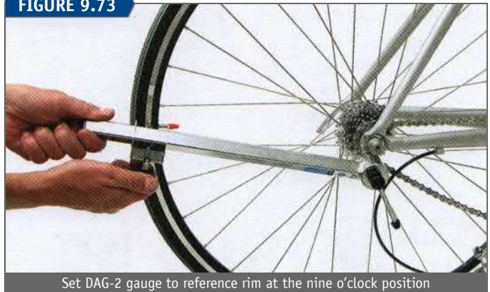
Set DAG-2 gauge to reference rim at the nine o'clock position
