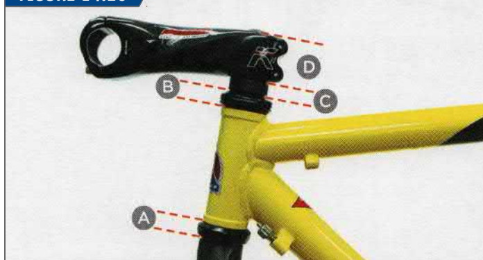
Stack height is composed of: (A) lower stack height, (B) upper stack height & (C) any spacers. Stem height (D) not included by headset manufacturers.
