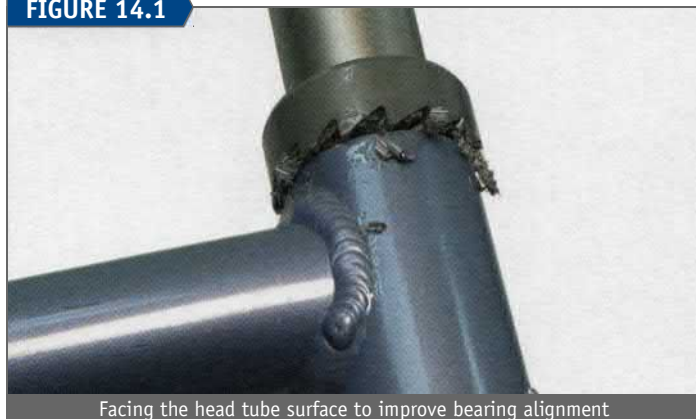
Facing the head tube surface to improve bearing alignment
