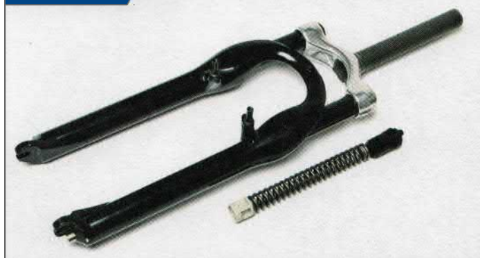
Helical compression spring from a shock fork
