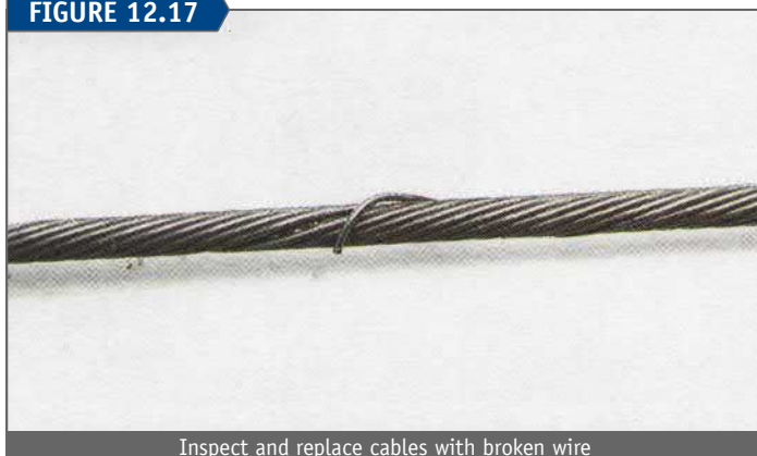
Inspect and replace cables with broken wire
