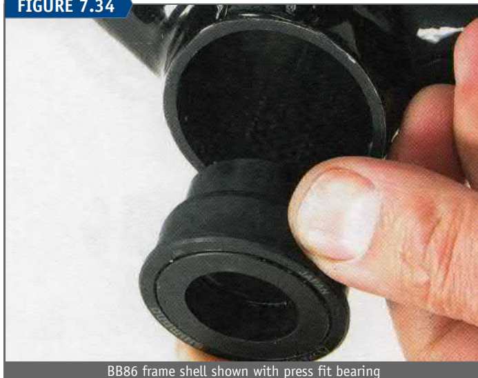
BB86 frame shell shown with press fit bearing
