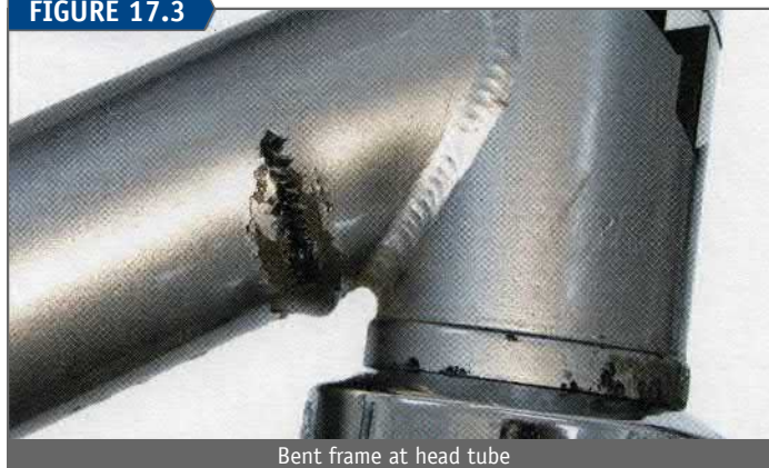
Bent frame at head tube
