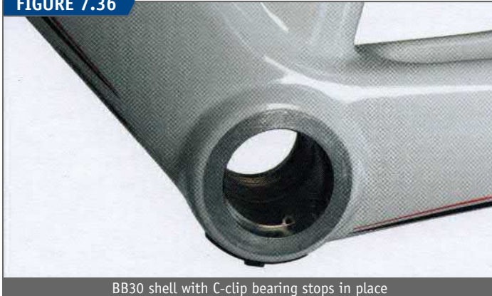
BB30 shell with C-clip bearing stops in place
