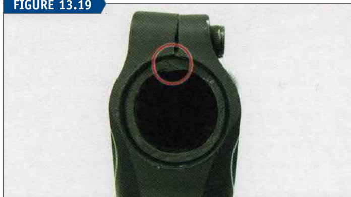
Cracked steering column from stem binder bolts
