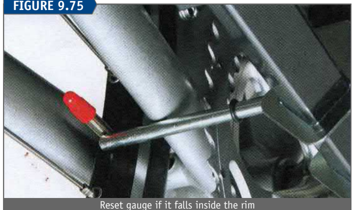
Reset gauge if it falls inside the rim
