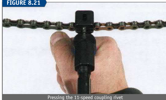
Pressing the 11-speed coupling rivet
