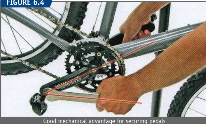
Good mechanical advantage for securing pedals
