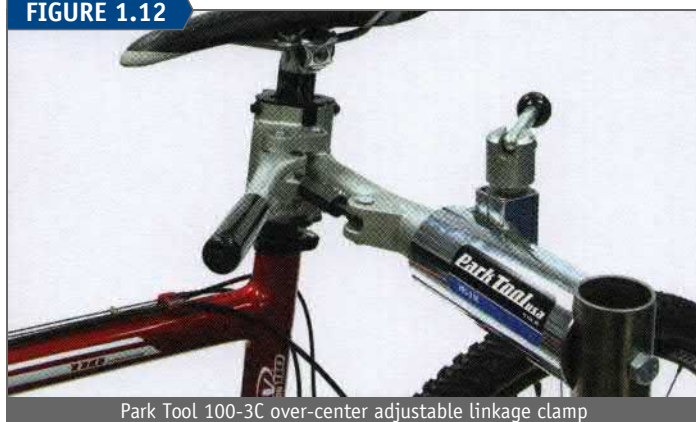
Park Tool 100-3C over-center adjustable linkage clamp
