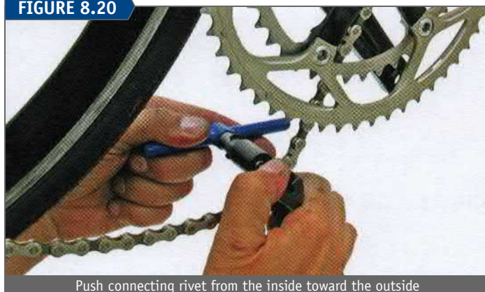
Push connecting rivet from the inside toward the outside
