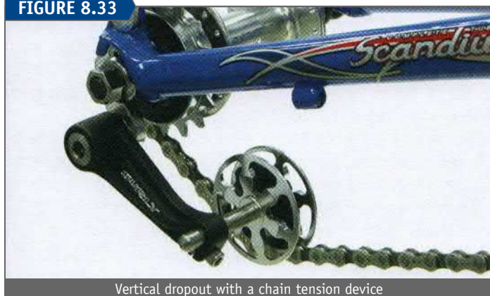
Vertical dropout with a chain tension device
