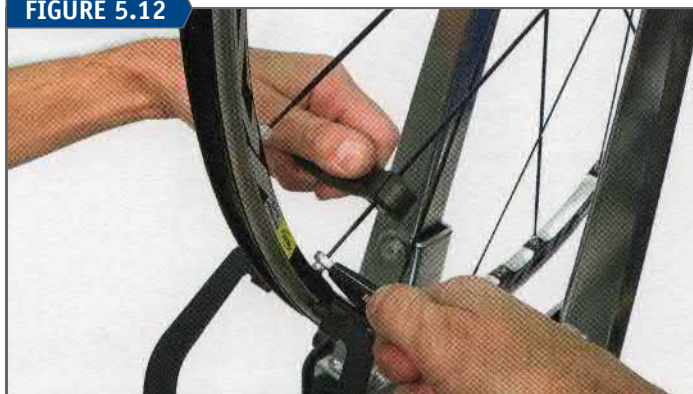
Use of the Park Tool BSH-1 to prevent bladed spoke twists
