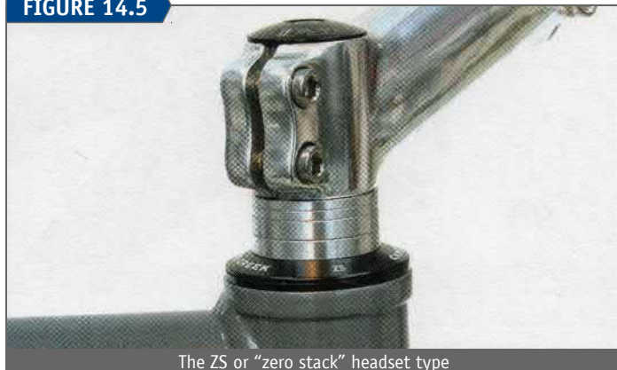
The ZS or "zero stack" headset type
