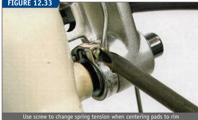
Use screw to change spring tension when centering pads to rim
