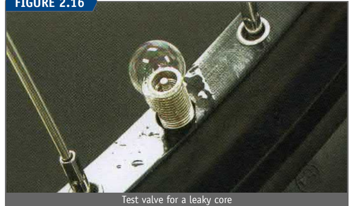
Test valve for a leaky core
