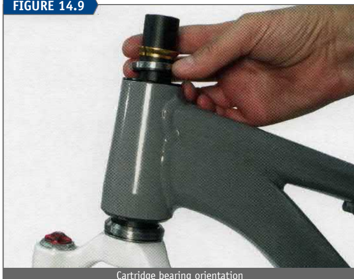
Cartridge bearing orientation
