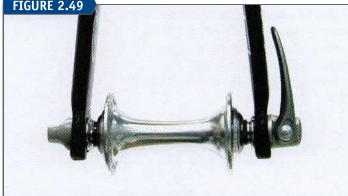
Closed skewer lever should be parallel to center plane of bike
