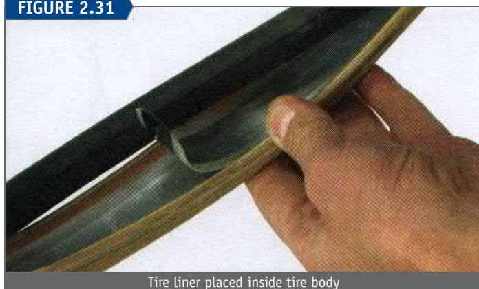
Tire liner placed inside tire body
