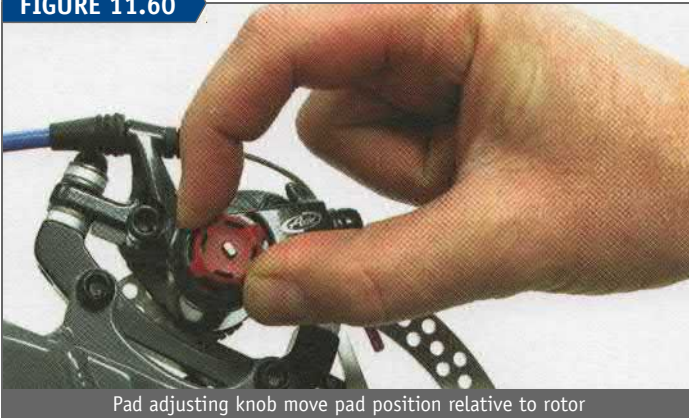
Pad adjusting knob move pad position relative to rotor
