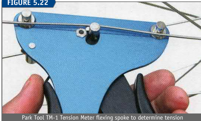
Park Tool TM-1 Tension Meter flexing spoke to determine tension
