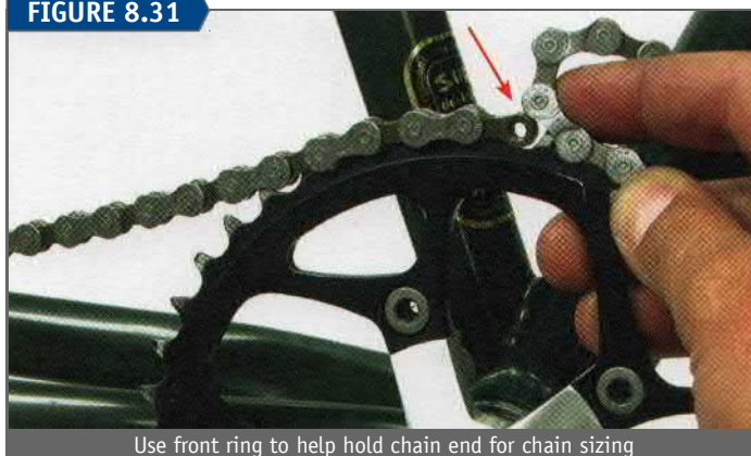
Use front ring to help hold chain end for chain sizing
