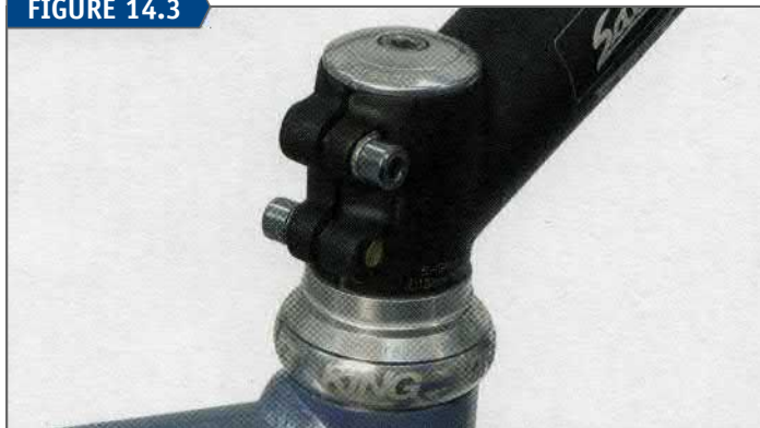
Threadless headset with external pressed cups, threadless stem, and top cap
