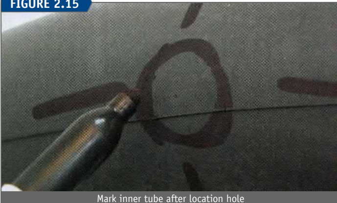
Mark inner tube after location hole
