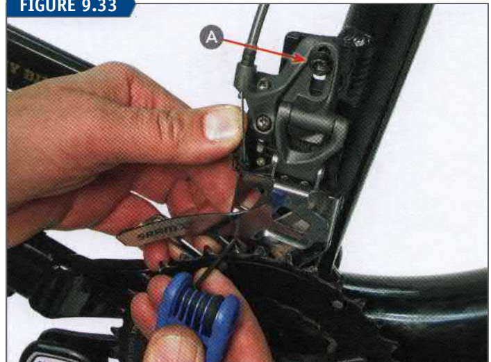
Checking a direct mount derailleur height using a 2.5mm hex wrench. A single bolt permits height changes (A).
