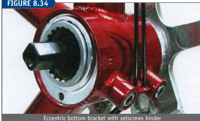
Eccentric bottom bracket with setscrews binder
