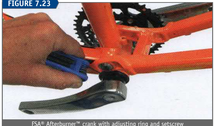
FSA® Afterburner™ crank with adjusting ring and setscrew
