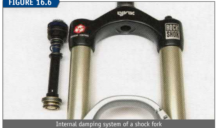
Internal damping system of a shock fork
