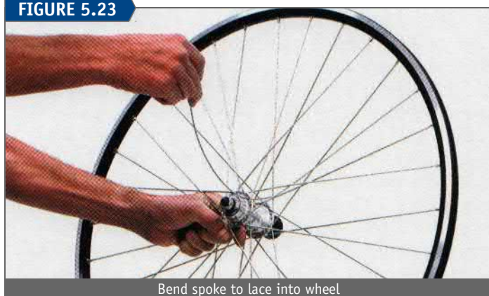
Bend spoke to lace into wheel
