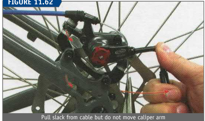
Pull slack from cable but do not move caliper arm
