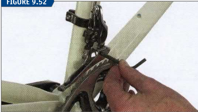
Position the outer cage flush with the straightedge using the L-limit screw
