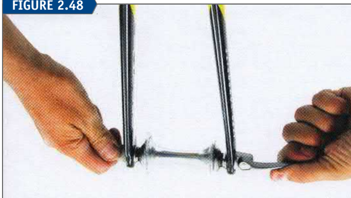
Adjust nut for lever resistance half way through swing
