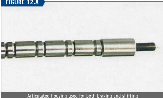
Articulated housing used for both braking and shifting
