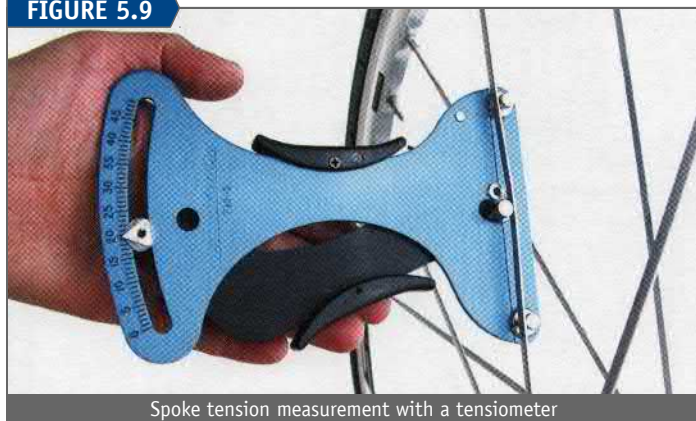
Spoke tension measurement with a tensiometer
