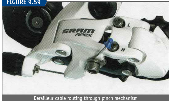
Derailleur cable routing through pinch mechanism
