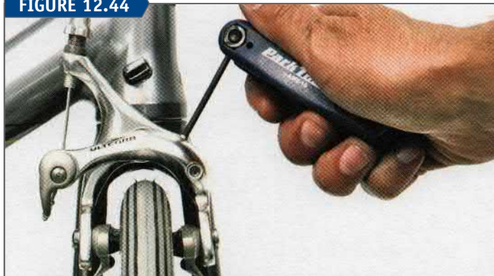
Center pads to rim with setscrew in brake bridge.
