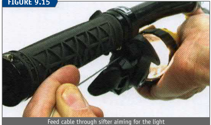
Feed cable through shifter aiming for the light
