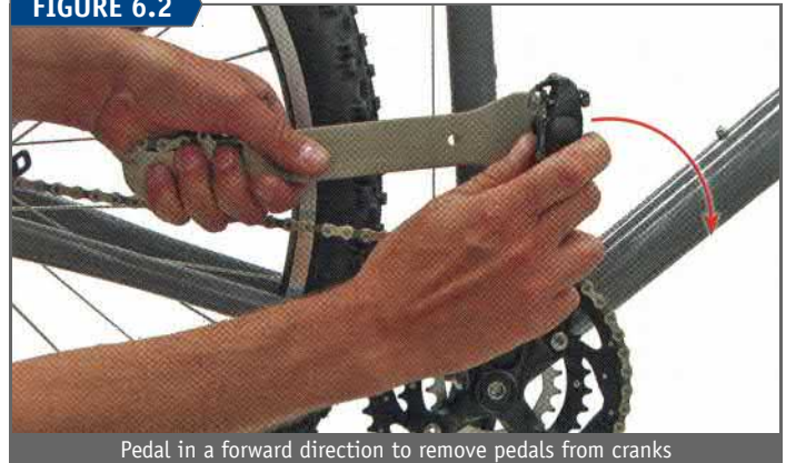
Pedal in a forward direction to remove pedals from cranks
