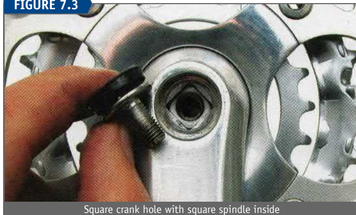
Square crank hole with square spindle inside
