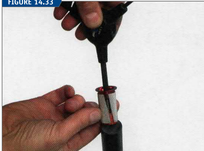
Install compression plug and secure into fork column
