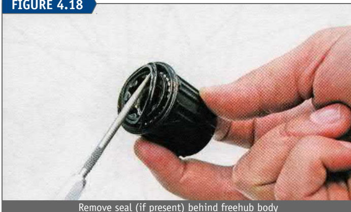
Remove seal (if present) behind freehub body
