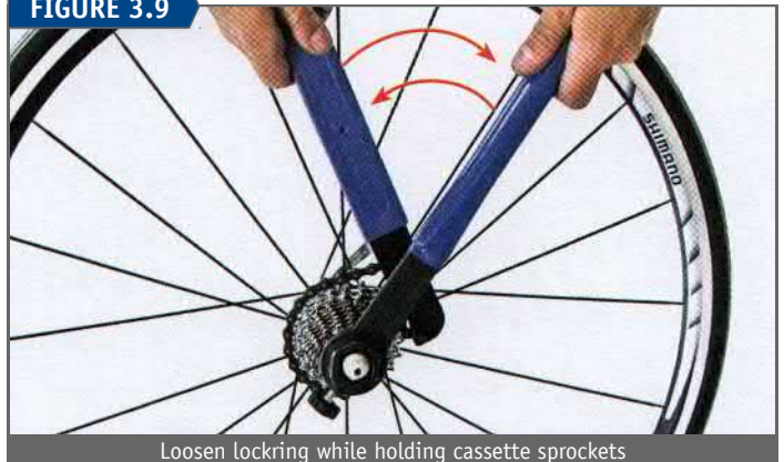
Loosen locking while holding cassette sprockets
