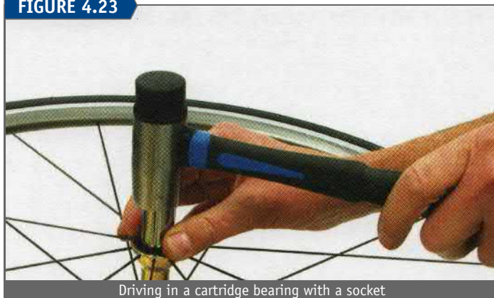
Driving in a cartridge bearing with a socket
