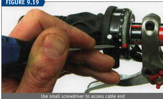
Use small screwdriver to access cable end
