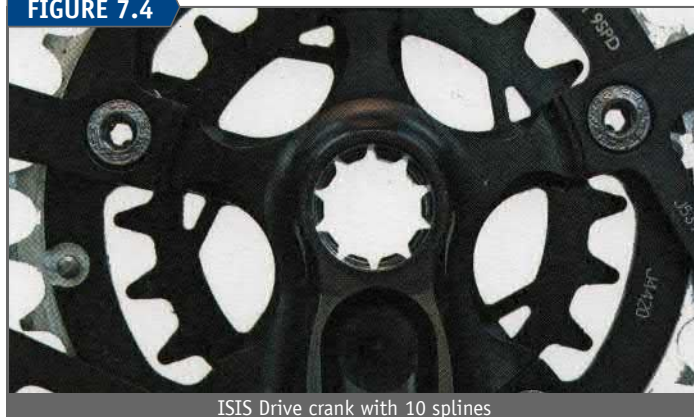
ISIS Drive crank with 10 splines
