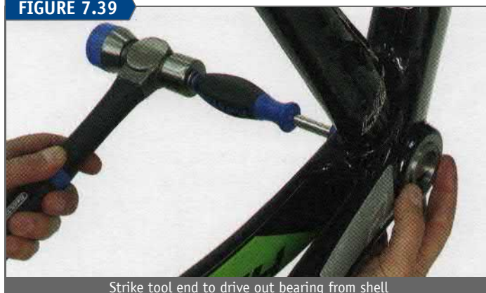
Strike tool end to drive out bearing from shell
