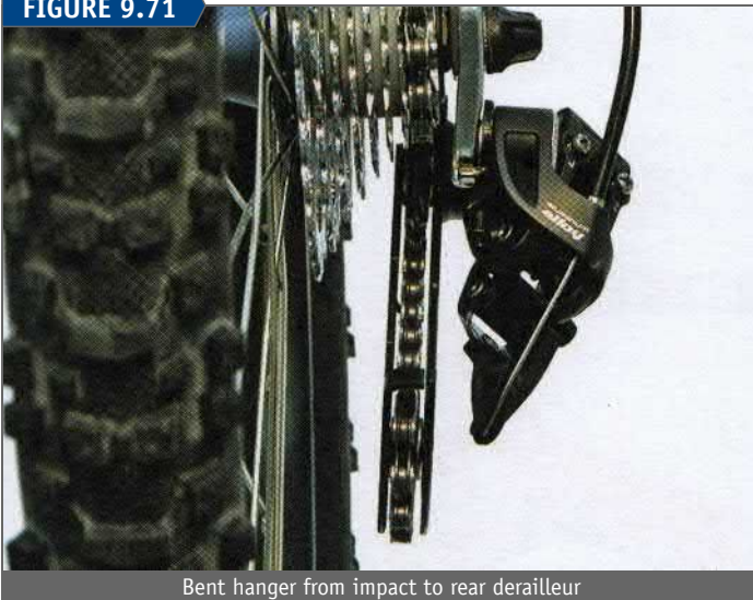
Bent hanger from impact to rear derailleur
