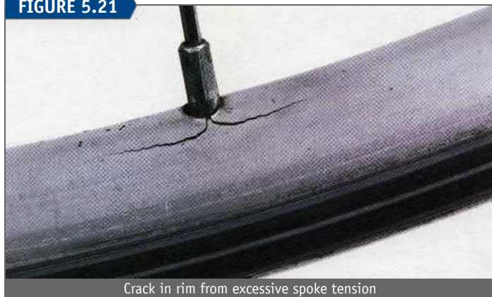
Crack in rim from excessive spoke tension
