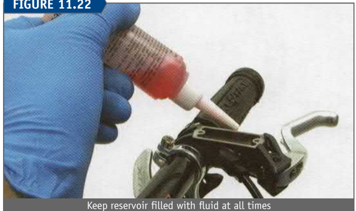
Keep reservoir filled with fluid at all times
