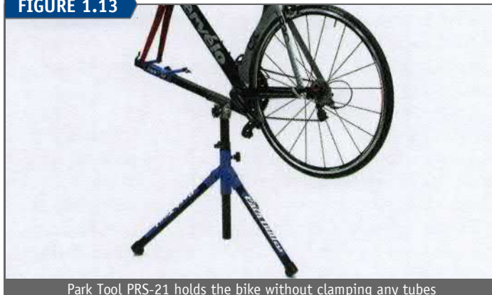
Park Tool PRS-21 holds the bike without clamping any tubes
