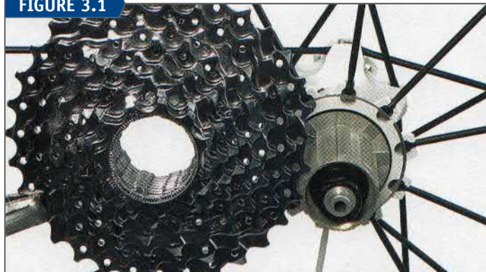
Cassette sprockets on the left with freehub body on the right
