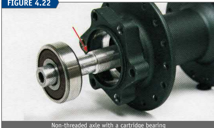
Non-threaded axle with a cartridge bearing
