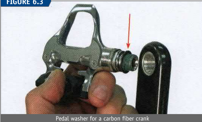
Pedal washer for a carbon fiber crank
