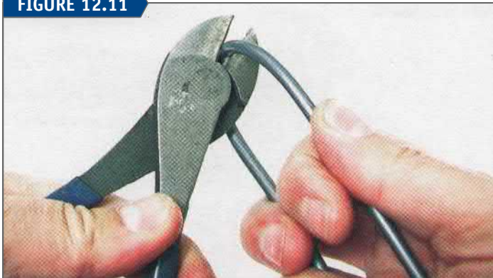
Flex the wound-type housing to open coils for side cutters
