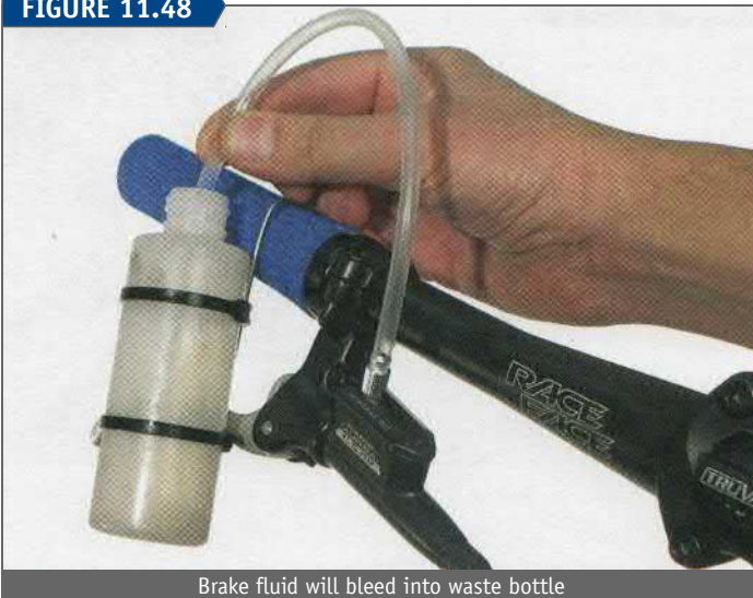
Brake fluid will bleed into waste bottle
