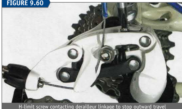
H-limit screw contacting derailleur linkage to stop outward travel
