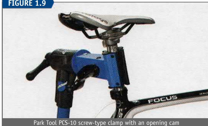
Park Tool PCS-10 screw-type clamp with an opening cam
