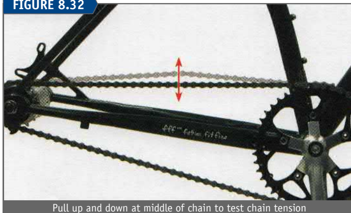
Pull up and down at middle of chain to test chain tension
