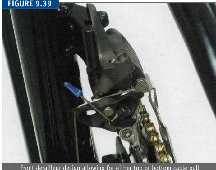
Front derailleur design allowing for either top or bottom cable pull
