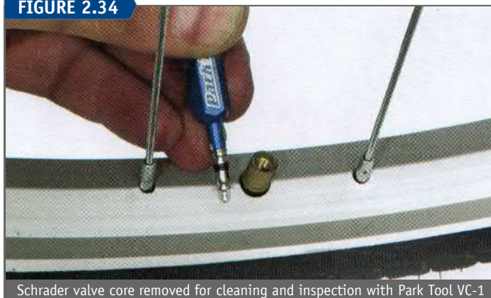
Schrader valve core removed for cleaning and inspection with Park Tool VC-1
